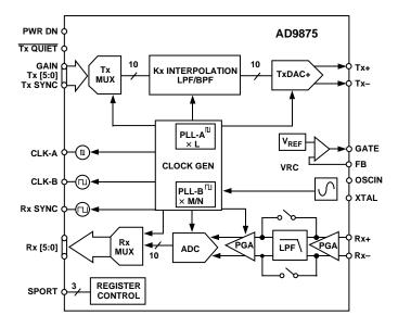
The receive path LPF cutoff frequency can be programmed to either 12 MHz or 26 MHz. The filter cutoff frequency can also be tuned or bypassed where filter requirements differ. The 10-bit ADC uses a multistage differential pipeline architecture to achieve excellent dynamic performance with low power consumption.
