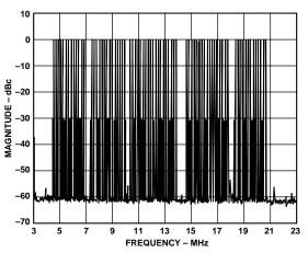
TPC 15. "In Band" Multitone Spectral Plot @  $f_{DATA} = 50$  MSPS,  $f_{OUT} = k \times 195$  kHz, 2× LPF
