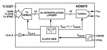
Figure 1. Transmit Path Block Diagram
