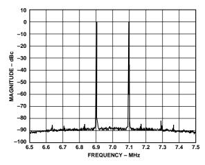
TPC 11. Dual Tone Spectral Plot @  $f_{DATA}$  = 32 MSPS,  $f_{OUT}$  = 6.9 MHz and 7.1 MHz, 4× LPF
