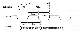
Figure 8. Timing Diagram Register Write to AD9875/AD9876
