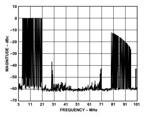
TPC 16. "Wide-Band" Multitone Spectral Plot @  $f_{DATA} = 50$  MSPS,  $f_{OUT} = k \times 195$  kHz,  $2 \times LPF$
