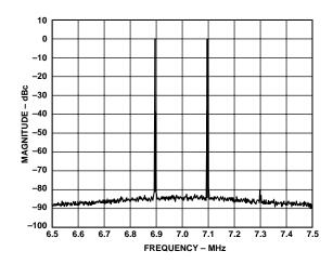
TPC 12. Dual Tone Spectral Plot @  $f_{DATA} = 50$  MSPS,  $f_{OUT} = 6.9$  MHz and 7.1 MHz, 2× LPF
