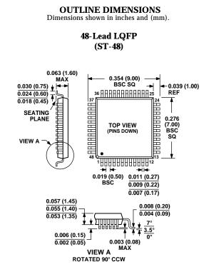
CONTROLLING DIMENSIONS ARE IN MILLIMETERS.
